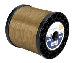
Axiom X-T coated wire is made a under private label for Single Source Technologies by one of the global leaders that manufacture coated EDM wires in France. It is a fast and precise wire recommended for Charmilles machines with older generators using X technology. It is particularly suited for precision as well as high-speed cutting. Axiom X EDM wire features a pure copper core with a CuZn50 (50% copper, 50% zinc) brass coating. Its tensile strength is 450 N/mm2.
